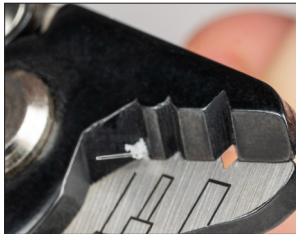
STEP 5 Carefully remove coating using Hole 3 on JIC-375.
