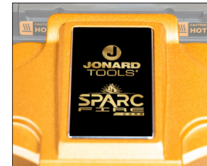
STEP 4 Gently close the Fusion Chamber cover. Splicing happens automatically.
