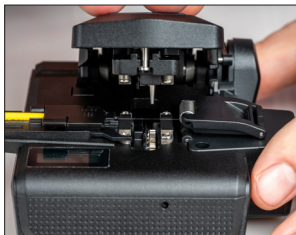
STEP 7 Place fiber in the correct channel for your fiber size, exposed fiber end should be in the automatic trash can, close lid to cleave. (Check manual for more information)
