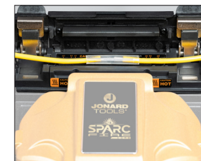
STEP 5 Slide the sleeve over the splice and place it in the heater.
